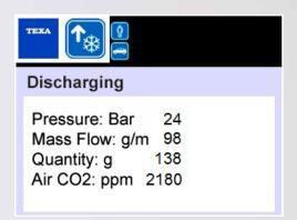
During refrigerant release, the display shows the quantity of refrigerant released and the pressure remaining in the system.
