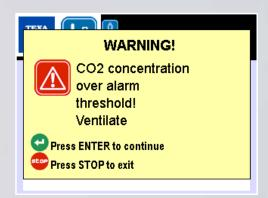
TEXA's operating software also warns you if the atmosphere in the work area becomes unsafe as a result of the release of CO<sub>2</sub>.
