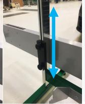
Continuous and spring-supported height adjustment of the cross member. The height of the cross member can now be adjusted by a single person. By adding 10 cm to the maximum height setting, vehicles with larger wheels (SUVs) can also be calibrated.
