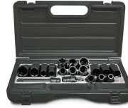
SK4M18N SK4M18N 1/2" Impact socket set (18 pcs) (10, 11, 13, 14, 17, 19, 21, 22, 24, 13L, 14L, 21L, 24L, 17L, 19L and 21L mm, extension 125 mm)
