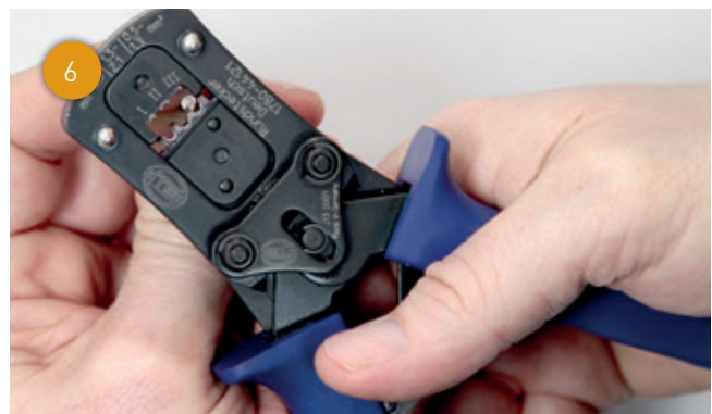
6 ... and place the plug flush with the front side in the pliers.
