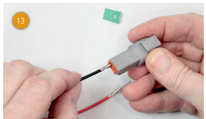
...and insert these also through the rubber seal of the housing until they audibly click into place.
