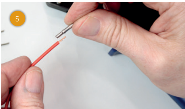
5 First, strip the vehicle cable to a maximum of 3-5 mm with a suitable tool...
