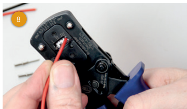
8 ... to crimp the contact sleeve with the cable.
