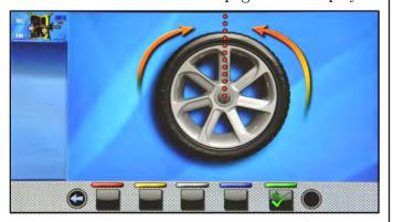
Bring any spoke upwards at "12 o'clock" position and
