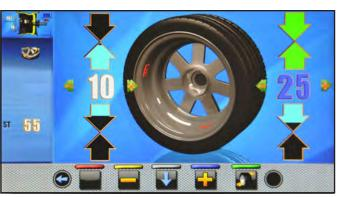
Fit the clip weight of the chosen value at 12 o'clock
