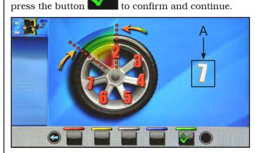
Lead to "12 hours" the 2nd spoke. The machine will automatically calculate the total number of spokes. If the value shown on the screen (A) is correct, press the
