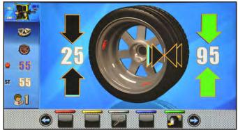
It is possible to fit a single weight at a predetermined distance from the machine, so as to optimize the weight consumption and reduce both the DYNAMIC and any remaining STATIC unbalance as much as possible. Unlike the standard STATIC procedure, the ECO-WEIGHT procedure, though only using one weight, also considerably reduces the DYNAMIC unbalance, because the fitting distance of the weight on the rim is also calculated.
