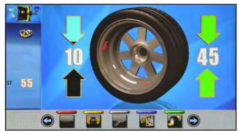
Once detected the unbalance values, verify that the machine displays the ability to use the "SPLIT" option
