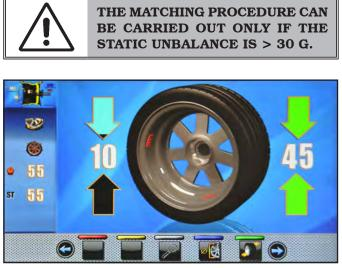
Once detected the unbalance values, verify that the machine displays the ability to use the "matching" options (**Fig. 52 ref. 4a**).
