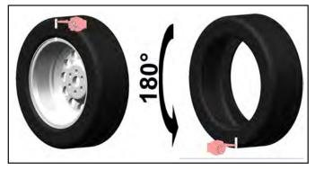
Fit the wheel back on the wheel balancer, positioning the reference mark on the rim in line with the arrow on the flange.
