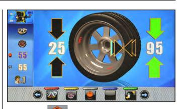
Press button **to** select such procedure and bring automatically the wheel into weight fitting position.
