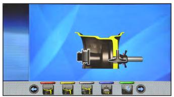
Place the distance-diameter caliper grippers (Fig. 49 **ref.** 1) on the inner side of the rim, as shown in Fig. 49.
