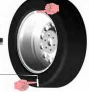
Position the tyre reference mark on the opposite side to the arrow on the flange
