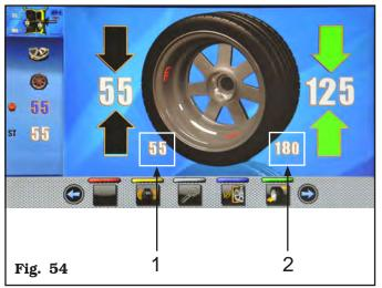
In this screen page, in addition to the information of the detected unbalance, there are measurements in mm where you must remove the gauge arm (Fig. 54 ref. 1-2) to apply the weights inside the rim.
