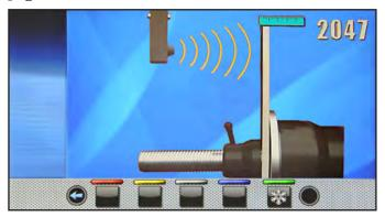
Close the wheel cover until bringing the automatic width sensor next to the sizing body previously installed.
