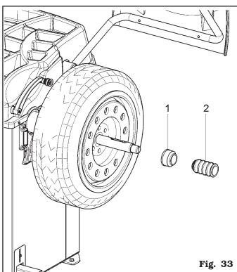
Lift the control pedal to close the mandrel and then clamp the wheel.
