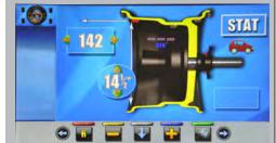
THIS CASE WILL OCCUR ONLY IF FROM "HOME" PAGE IS DETECTED ONLY ONE MEASUREMENT IN-SIDE THE RIM. THE PROGRAM WILL AUTOMATICALLY SET TO "STATIC" BUT IT WILL MAKE IT POSSIBLE (IN CASE OF ABSENCE OF EXTERNAL DATA GAUGE) TO MANUALLY ENTER RIM WIDTH AND TO QUICKLY SWITCH TO THE PROGRAM "DYNAMIC".
