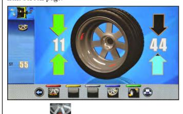
Press button to enter "SPLIT" function. On the monitor screen will be displayed where you must enter the value of the weights to be fitted.
