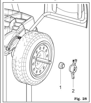
Some aluminium wheels, with very high centring, must be fitted with the cone outside the wheel.
