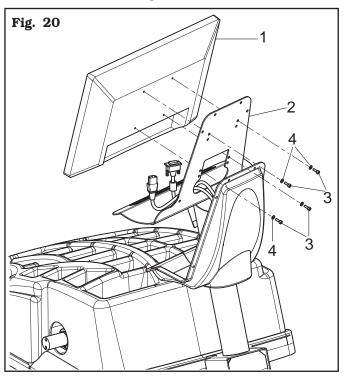
Mount the guard (Fig. 21 ref. 1) to the support (Fig. 21 ref. 2) with the 6 screws (Fig. 21 ref. 3) and the washers (Fig. 21 ref. 4) supplied.
