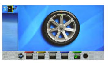
**STEP 1**. Move the slider on the flange to the "12 o'clock" position. Make a reference mark, using chalk for instance, on the rim and tyre, in line with the arrow on the flange, so as to be able to fit the rim back on in the same position on the machine.
