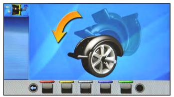
After having fitted wheel back in position, close the protection guard to make an automatic wheel spin. At the end of the spin the monitor will display the following screen:
