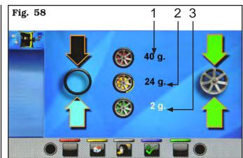
In this screen you will see the dynamic unbalance that the wheel had before performing the operation (**Fig. 58 ref. 1**), the dynamic unbalance after having rotated the tyre of  $180^{\circ}$  compared to the rim (**Fig. 58 ref. 2**) and the unbalance which can be obtained following the directions of the machine (**Fig. 58 ref. 3**).
