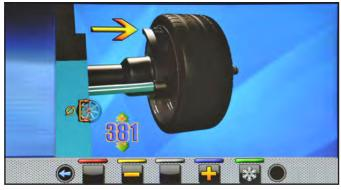
Measure the exact diameter of a rim (see Fig. 69) and place it on the screen on the monitor by pressing the
