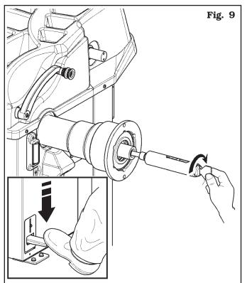
3. Fit the external mandrel and tighten it manually (**Fig. 10**).
