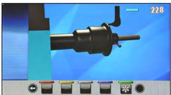
Move the tip of the width measuring device (**Fig. 73 ref. 1**) in line with the outer surface of the flange (**Fig. 73 ref. 2**).
