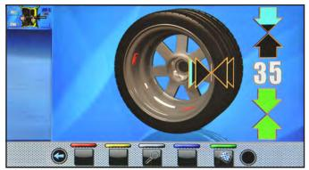
Extract the gauge rod, and fit the FIRST weight in the position shown by the machine, as explained in
