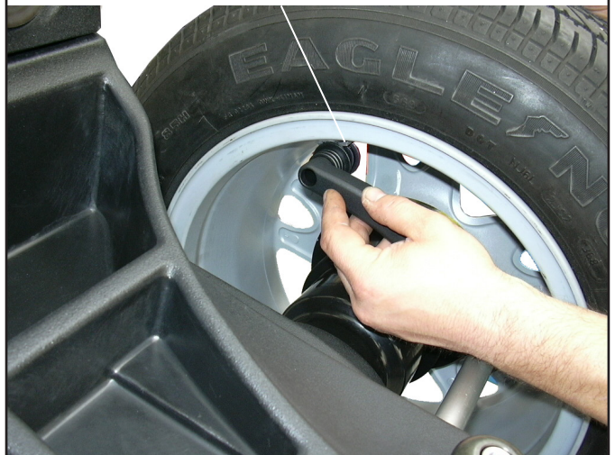
Fig. 49 Fit weight on the position where pliers touches the wheel
