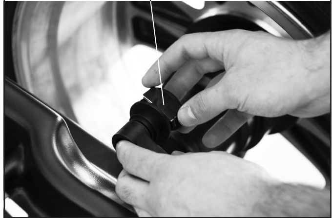
Fig. 48 Fit the adhesive weight in the pliers of the gauge rod
