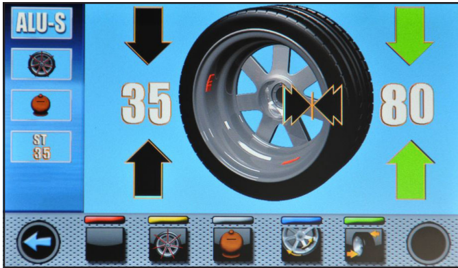
Fig. 48 Fit the adhesive weight in the pliers of the gauge rod
