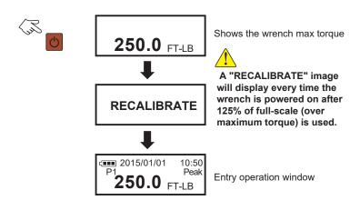
Turn Off- Press POWER button for 3 seconds.
