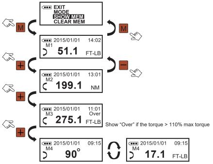
Exchange angle and torque values if using Angle Function
