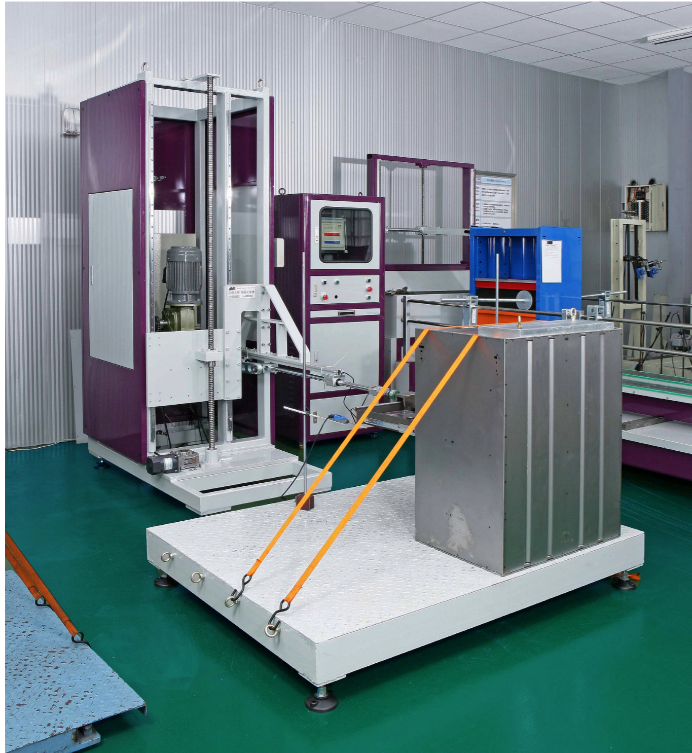
The drawers' strength, runners, closing and locking functions are tested through 50,000 opening and closing cycles with an applied load of 40 kg.
