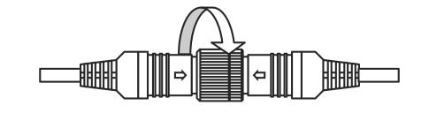
3. Tighten cable connection firmly in order to prevent water ingress.
