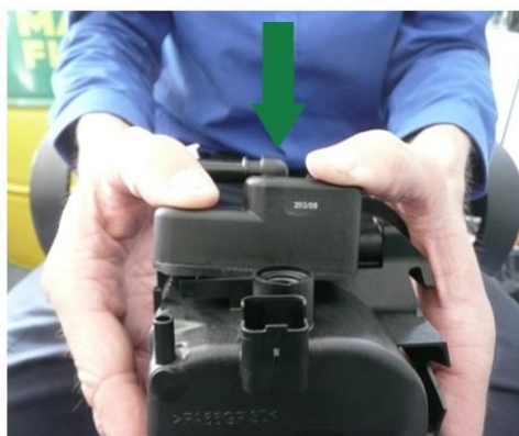
3 Use force of both thumbs to push the heater down until you hear a click
