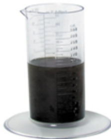
Contaminated system oil
