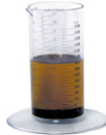
Contamination Deposit in the system's oil
