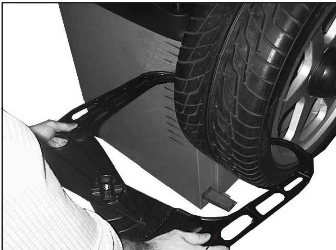
MANUAL EXTERNAL DATA GAUGE Rim width manual detection
