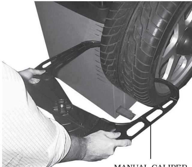
MANUAL CALIPER. Width manual detection
