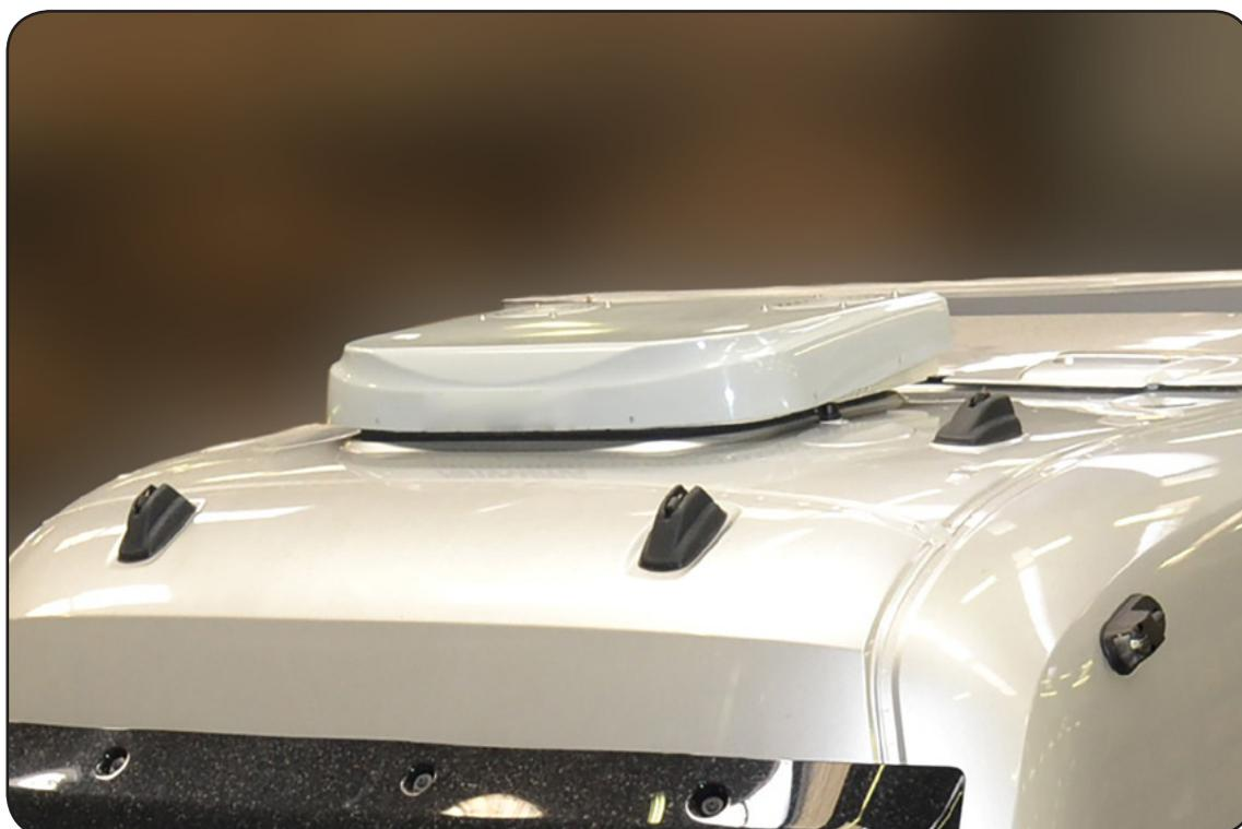
Fix the air conditioner using the brackets **B**: insert the ends of the brackets under the lining to gain a grip on the metal parts; insert screws **CC** with the washers **DD** and nuts **EE** and screw them into the threaded sockets on the bottom of the air conditioner. Tighten and then tighten the nuts **EE** against the brackets **B**.
