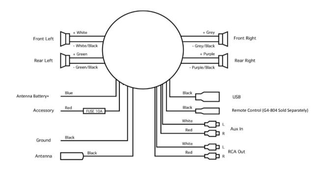
Connections to the various speaker and power wires should be soldered or crimped. They should be shrink wrapped to ensure protection from water damage.
