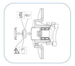
Dismount the old wheel brake disc, nut and mounting cap. Never re-use the old nut and cap.
