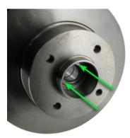
When installing the bearing and the brake disc, apply the force ONLY on the inner ring of the bearing.
