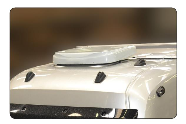
Fix the air conditioner using the brackets **B**: insert the ends of the brackets under the lining to gain a grip on the metal parts; insert screws **CC** with the washers **DD** and nuts **EE** and screw them into the threaded sockets on the bottom of the air conditioner. Tension and then tighten the nuts **EE** against the brackets **B**.
