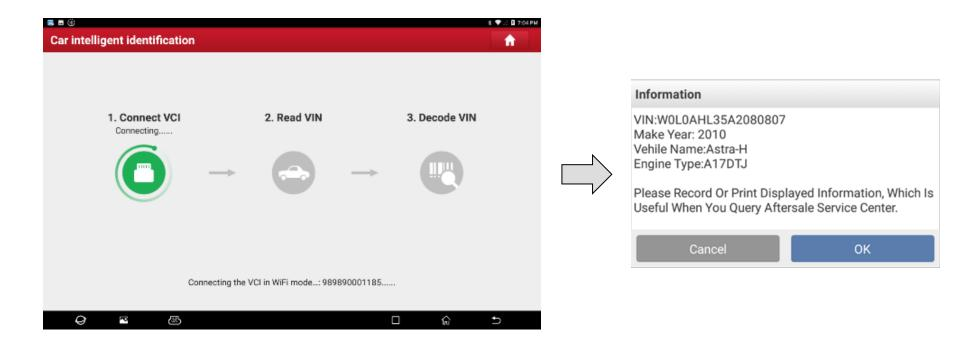
The vehicle model, manufacture year can be found automatically through the VIN number. This function is more convenient than manual selection.
