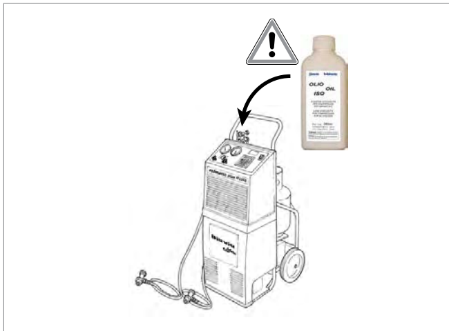
Fig. 50: Fill service station with oil
