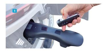
If the V2L-HK cuts-off power during use it may be due to an overload or low battery charge. Check the vehicle condition and charge level to determine why there is no output power.
