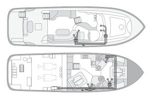
In this 40' motor yacht electrical fan blowers are used to heat up the boat. They are very compact and may be easily installed in small spaces, blowing hot air through air ducts into each cabin. The windscreen has a separate blower to demist and defrost.
