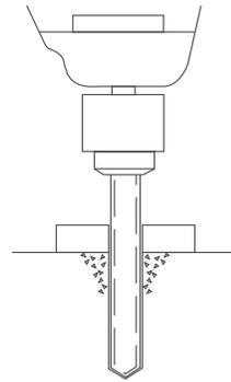
Drill holes using correct carbide tipped masonry bit drill bit.
