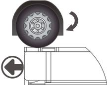
Always make sure the bolts stop extension out while vehicle drive onto the lift.
