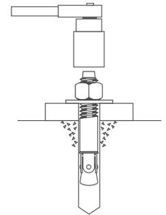
Tighten nut with torque wrench. For chemical anchor bolts read the manual of the anchor manufacturer.
