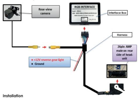
NB: Before installation, switch off ignition, disconnect the vehicle battery and remove the vehicle's head unit.
