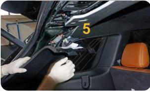
5. To remove left D-column trim, loosen safety dog first
