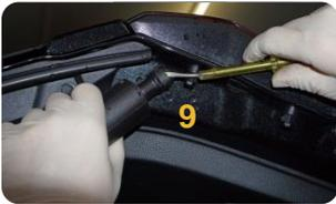
9. With a suitable tool, loosen safety clip from drive's ball pivot seat at the tailgate and remove
