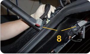
8. Remove Powerise drive connector from plug connection and carefully guide out of cable routing
