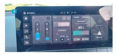
If the V2L-MG cuts-off power during use it may be due to an overload or low battery charge. Check the vehicle condition and charge level to determine why there is no output power.
