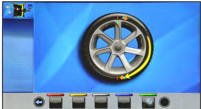
**STEP 2.** Remove the wheel from the wheel balancer. Remove the tyre and turn it on the rim through 180°.
