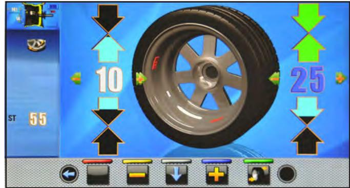
Fit the clip weight of the chosen value at 12 o'clock
