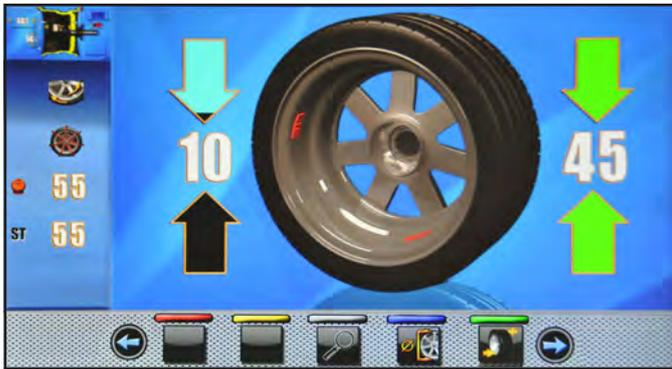
Once detected the unbalance values, verify that the machine displays the ability to use the "matching" options (Fig. 52 ref. 4a).
