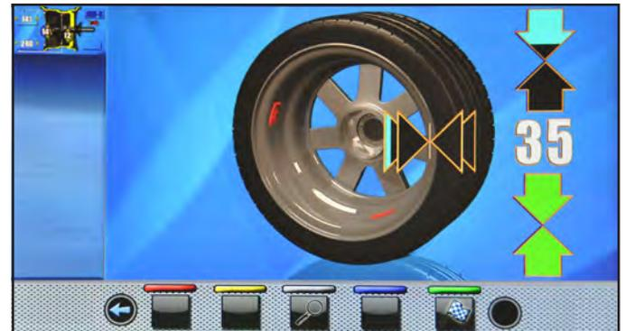
Extract the gauge rod, and fit the FIRST weight in the position shown by the machine, as explained in
