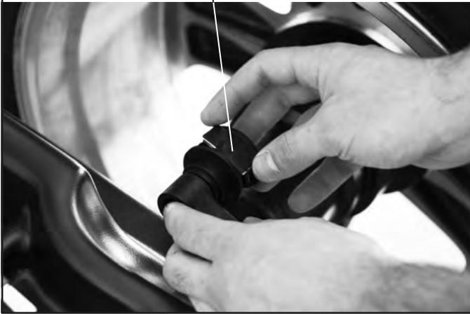
2. Pull out the gauge until the arrows (**Fig. 52 ref. 6**) both turn green.
