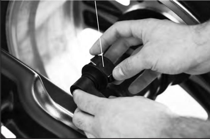
Pull out the gauge rod until the arrows (**Fig. 55 ref. 6**) turn green.
