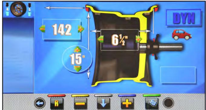
**PRESS THE BUTTON** **(Fig. 40 ref. 1) TO DISABLE AUTOMATIC FUNCTION OF THE DISTANCE-DIAMETER CALIPER ARM WHEEL BALANCING SELECTION, DESCRIBED IN PAR. 14.2.1. TO BE ABLE TO REUSE THE AUTOMATIC FUNCTION TO SELECT THE WHEEL BALANCING PROGRAM WITH GAUGE ARM, IT IS NECESSARY TO RETURN TO "HOME" PAGE, BY PRESSING THE** **BUTTON**
