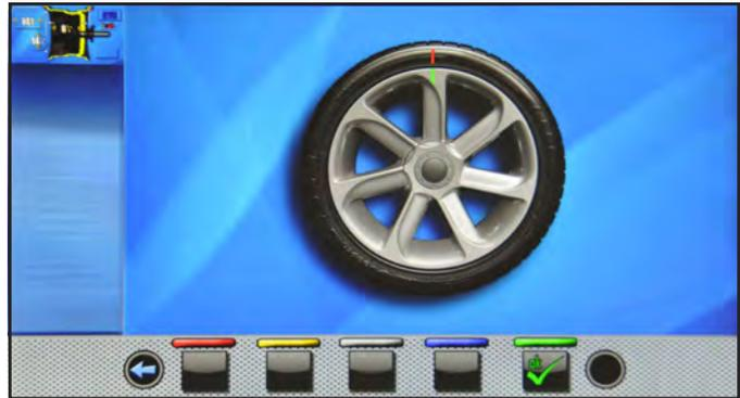
**STEP 1.** Move the slider on the flange to the "12 o'clock" position. Make a reference mark, using chalk for instance, on the rim and tyre, in line with the arrow on the flange, so as to be able to fit the rim back on in the same position on the machine.
