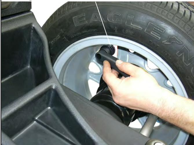
4. Bring the distance-diameter caliper arm into resting position.
