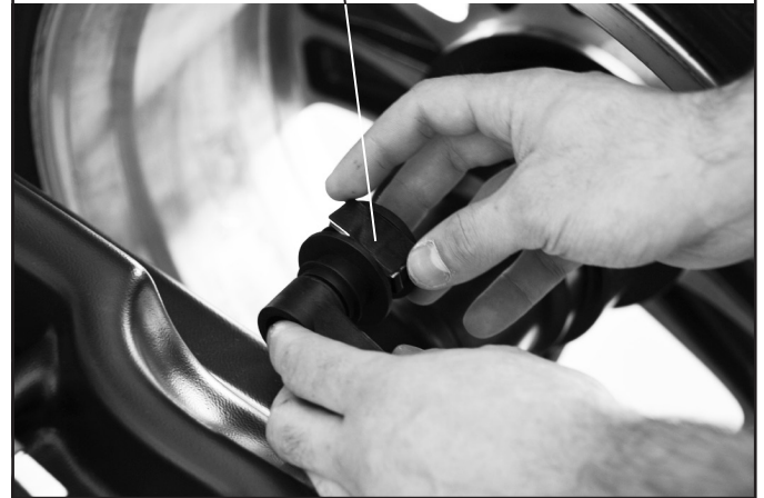
Fig. 35 Fit the adhesive weight in the pliers of the gauge rod
