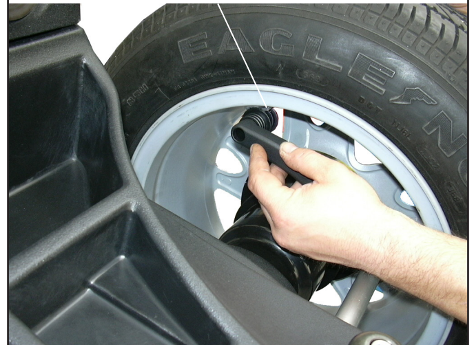
Fit weight on the position where pliers touches the wheel Fig. 36
