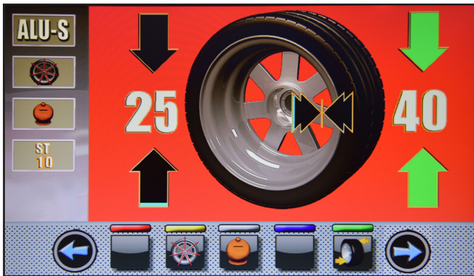
Fig. 35 Fit the adhesive weight in the pliers of the gauge rod
