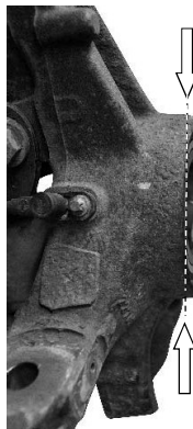
Fig. 46: Safety ring is fully engaged in the groove.
