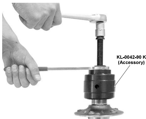
Fig. 38: Pull off inner bearing race, e.g. with the aid of KL-0042-90 K (accessory).
