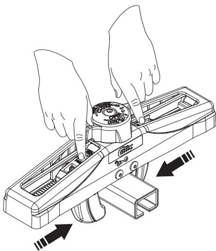
Push together until both hooks meet roofrack.
