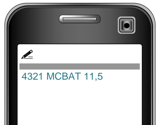
Example: Reset of the GPS locator to factory default setting
