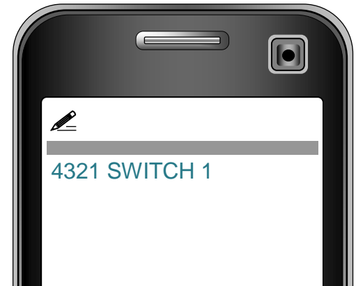
Example: Switching the relay
