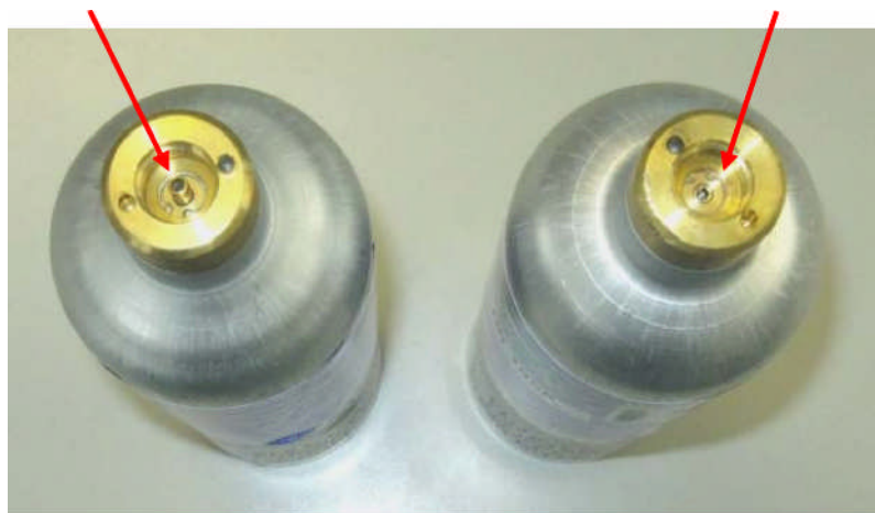
Testgas flaska med hel ventil / Test gas bottle with complete internal valve
