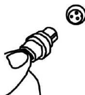
Fig. 8: Connect switch connector of wheel-guard cover
