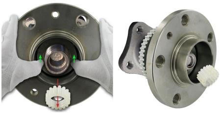
The plastic joining sleeve ring will be automatically pushed out by the axle stub, when mounting the bearing in a correct way, applying the force on the inner ring. Do not push out the plastic sleeve manually before mounting.
