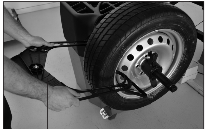
MANUAL CALIPER. Width manual detection
