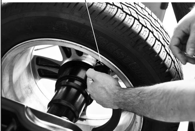
Fit weight on the position where pliers touches the wheel Fig. 54
