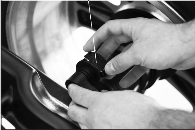
Fig. 53 Fit the adhesive weight in the pliers of the gauge rod
