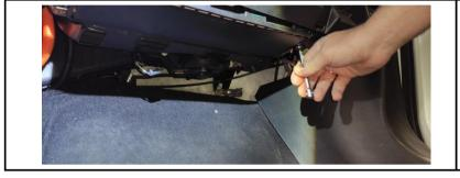
4. If equipped, remove the passenger knee airbag
