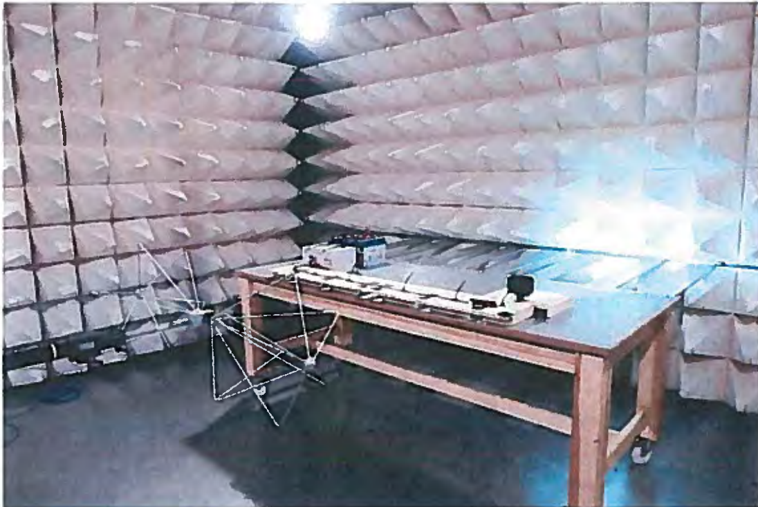
Photo 1: Test setup in the anechoic chamber, radiated emissions – ALSE method from 30 to 200 MHz
