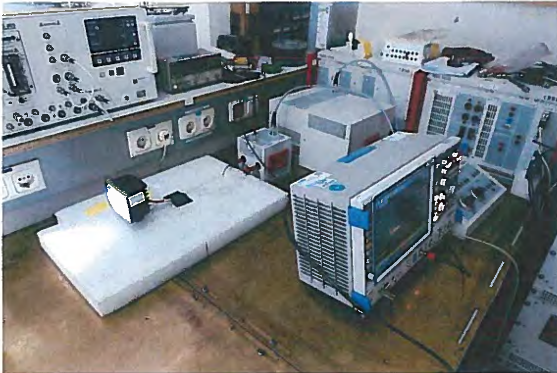
Photo 3: Test setup in the laboratory 2, conducted emissions – voltage transients
