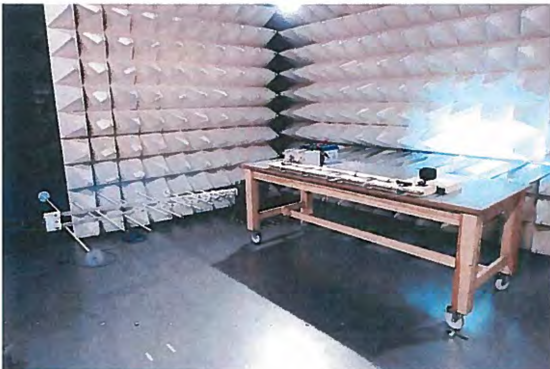
Photo 2: Test setup in the anechoic chamber, radiated emissions – ALSE method from 200 to 1000 MHz
