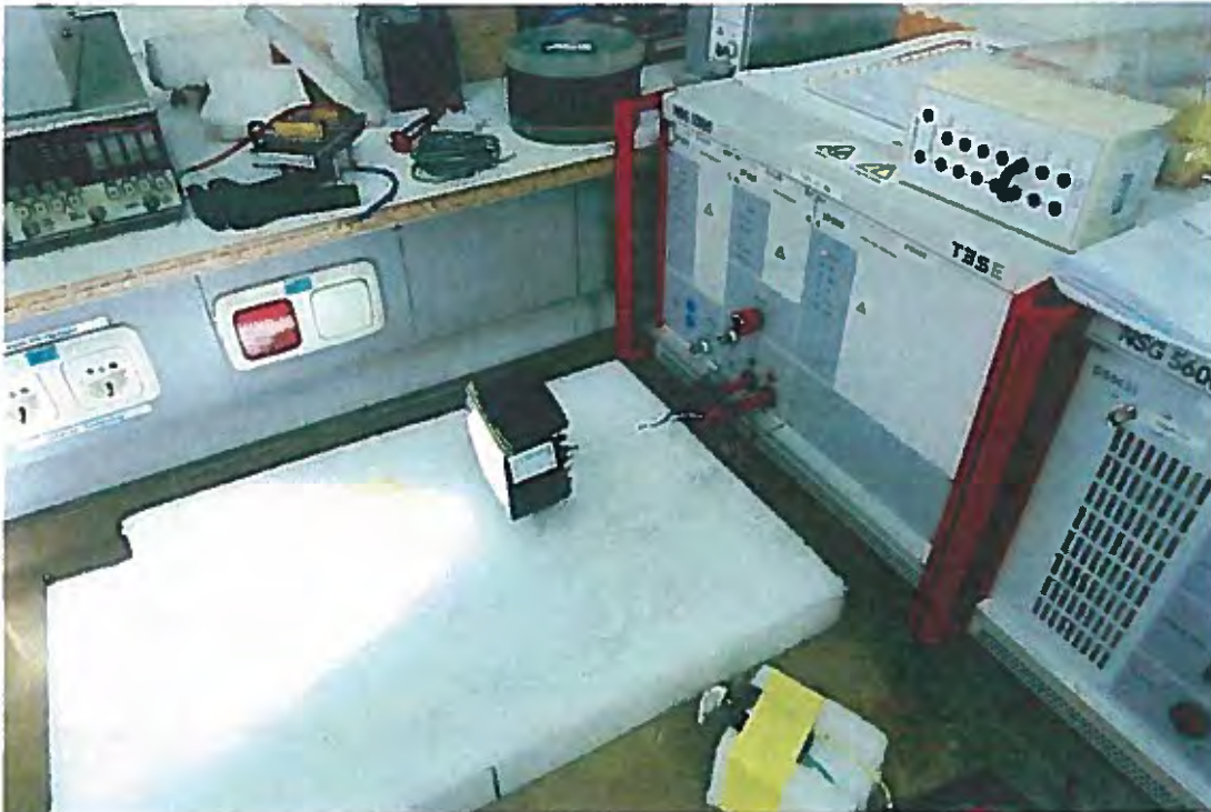
Photo 7: Test setup in the laboratory 2, Electrical transients conduction along supply lines only
