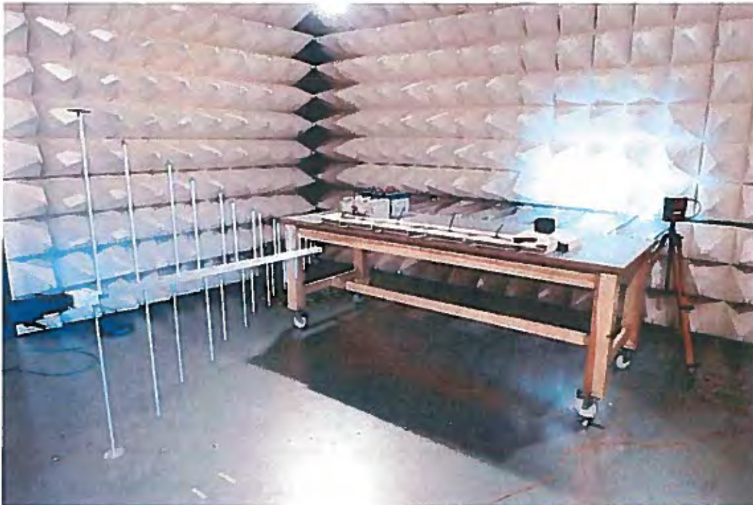
Photo 5: Test setup in the anechoic chamber, Radio-frequency electromagnetic fields – Absorber lined shielded enclosure (ALSE) from 400 to 1000 MHz
