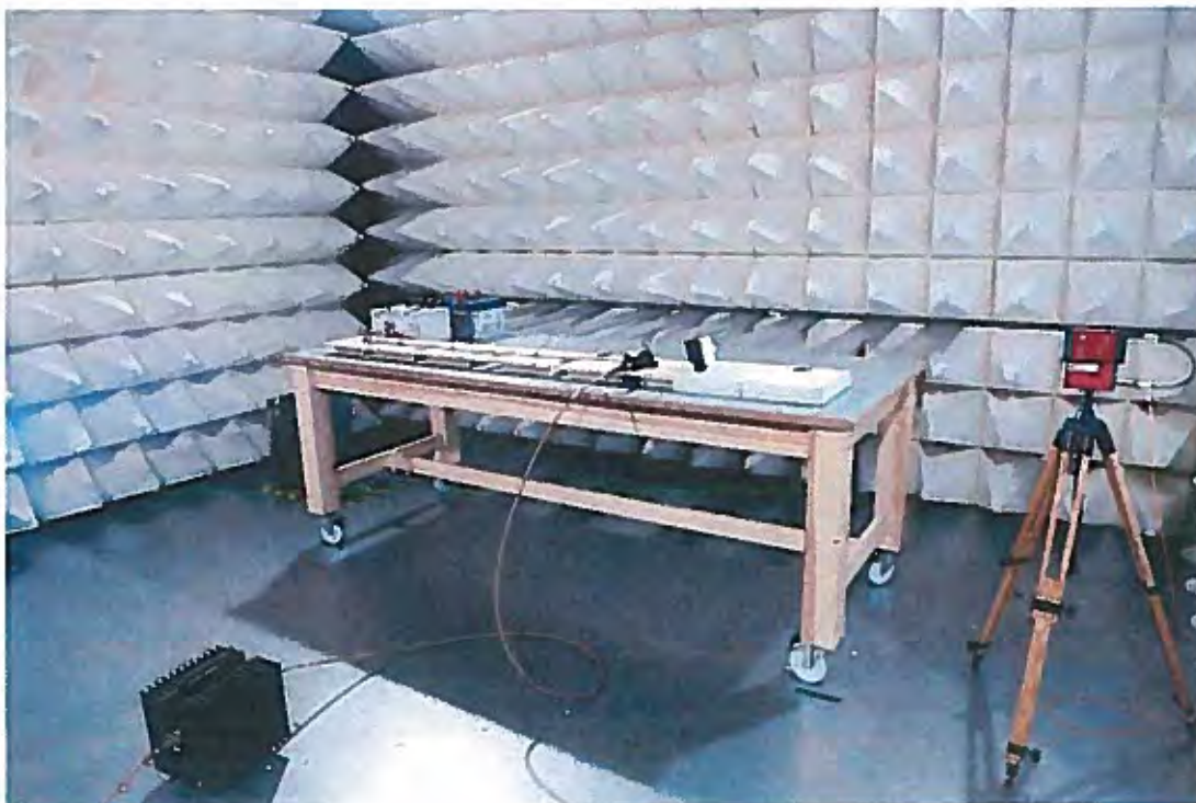
Photo 4: Test setup in the anechoic chamber, Bulk current injection (BCI) from 20 to 400 MHz
