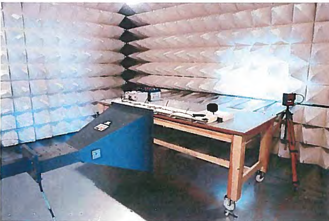
Photo 6: Test setup in the anechoic chamber, Radio-frequency electromagnetic fields – Absorber lined shielded enclosure (ALSE) from 1000 to 2000 MHz
